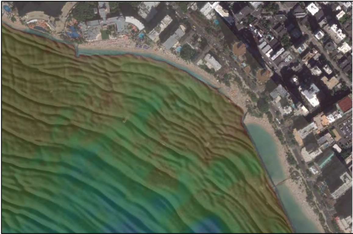
Figure 4-6 Water surface snapshot from BOUSS2D
