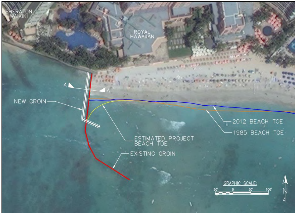
Figure 2-6 Concrete wall groin plan view
