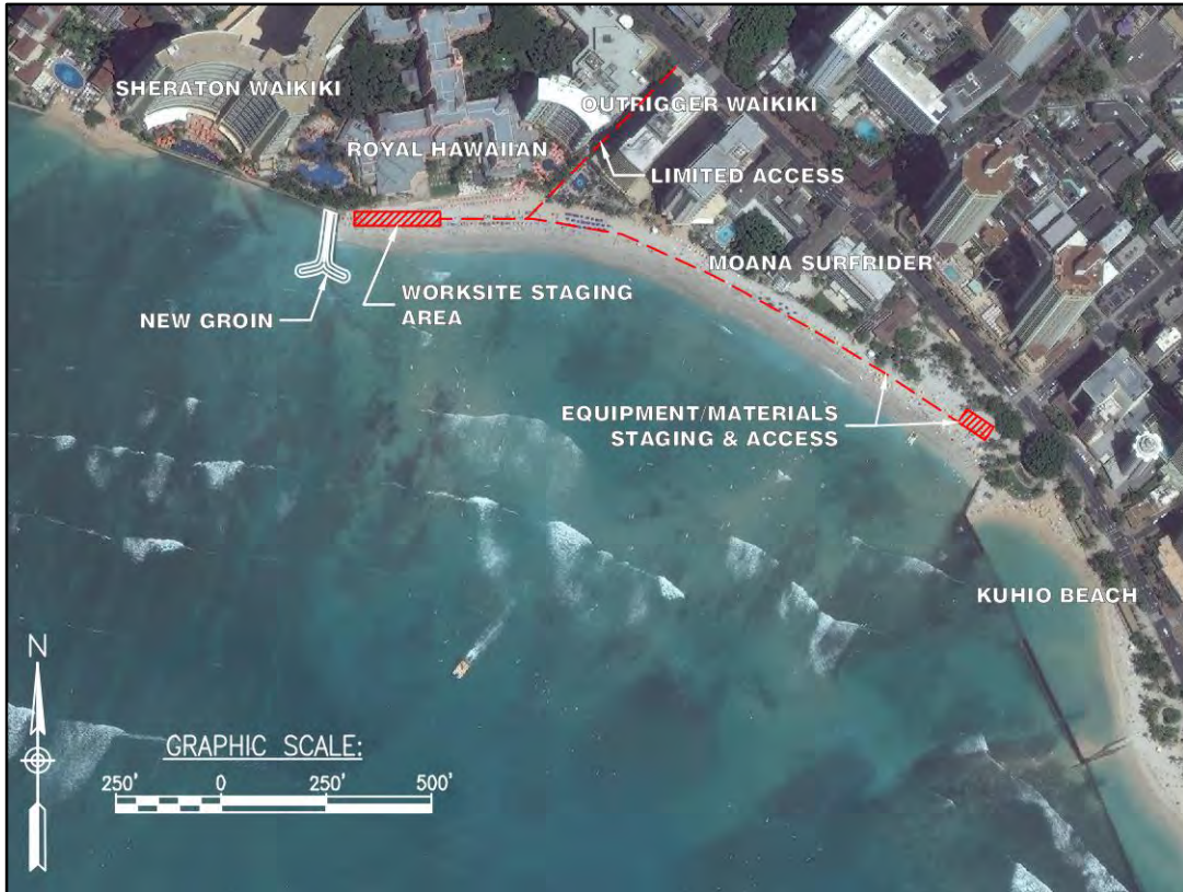
Figure 2-11 Construction access and staging areas
