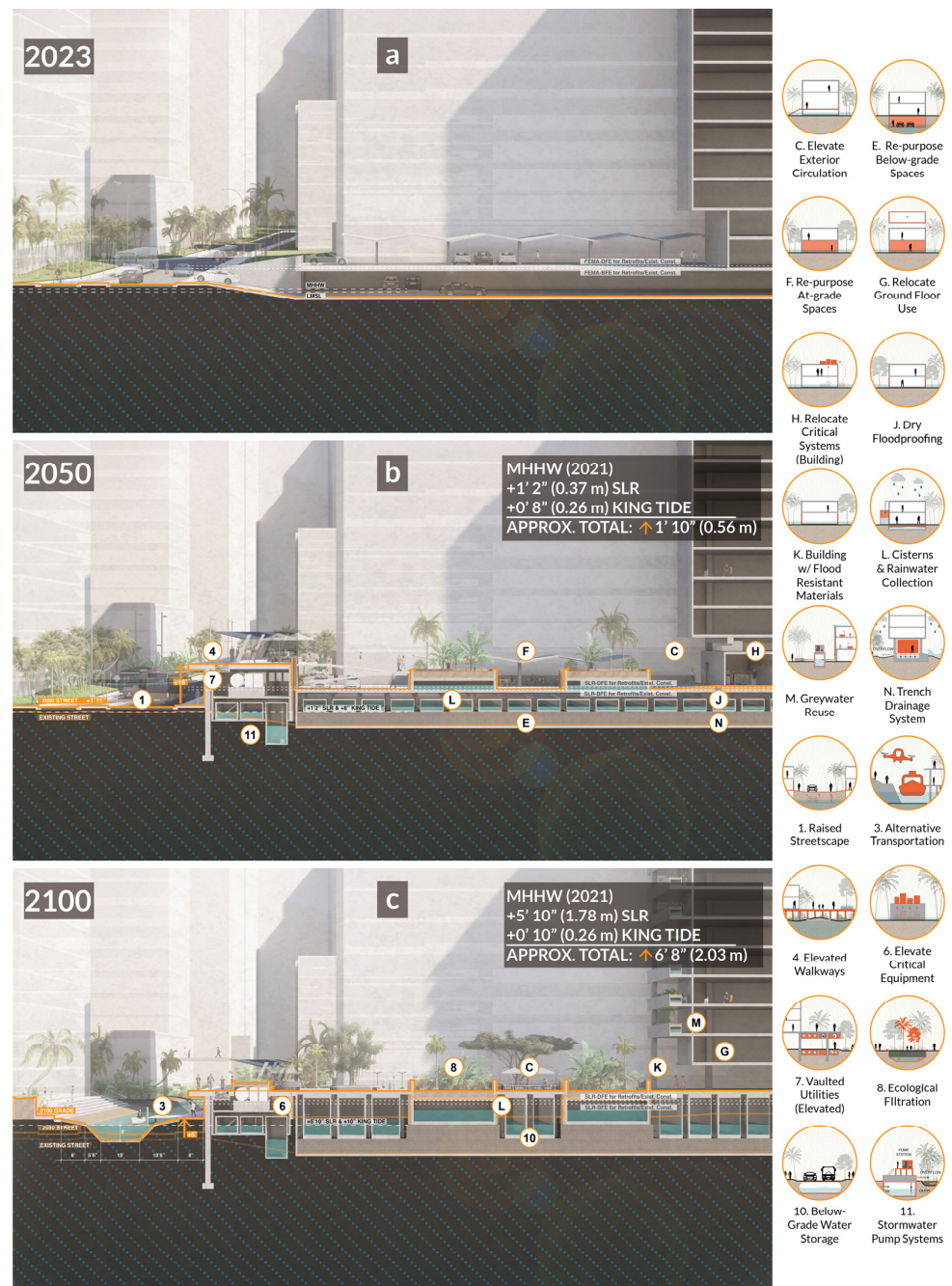
Figure 4. Building and street: (a) present conditions, (b) 2050 Adaptations, (c) 2100 Adaptations. Letters and numbers on the renderings correspond to the icons of adaptation strategies. Image credit: Eric Teeple.
