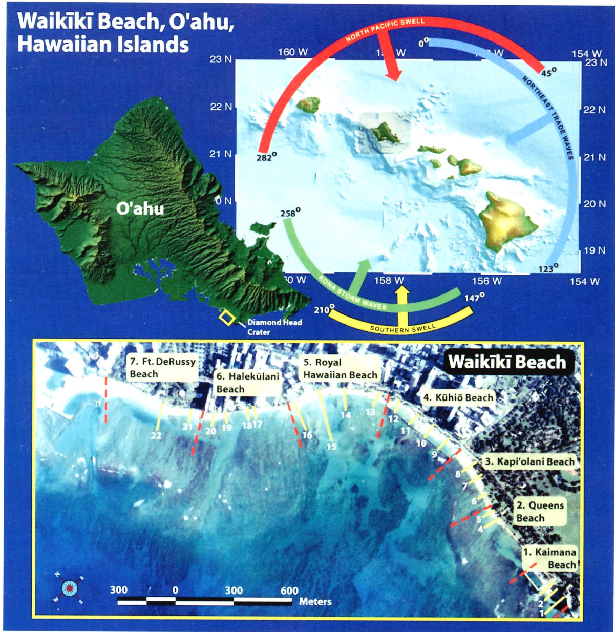
Figure 2. Map of the study area at Waikiki Beach, Oahu, Hawaii. Along the shoreline, physical structures create seven littoral cells. Beach profile locations are designated by yellow lines, labeled 1–22 from southeast to northwest. Profiles were surveyed approximately every other month for 20 months (October 2000–May 2002).
