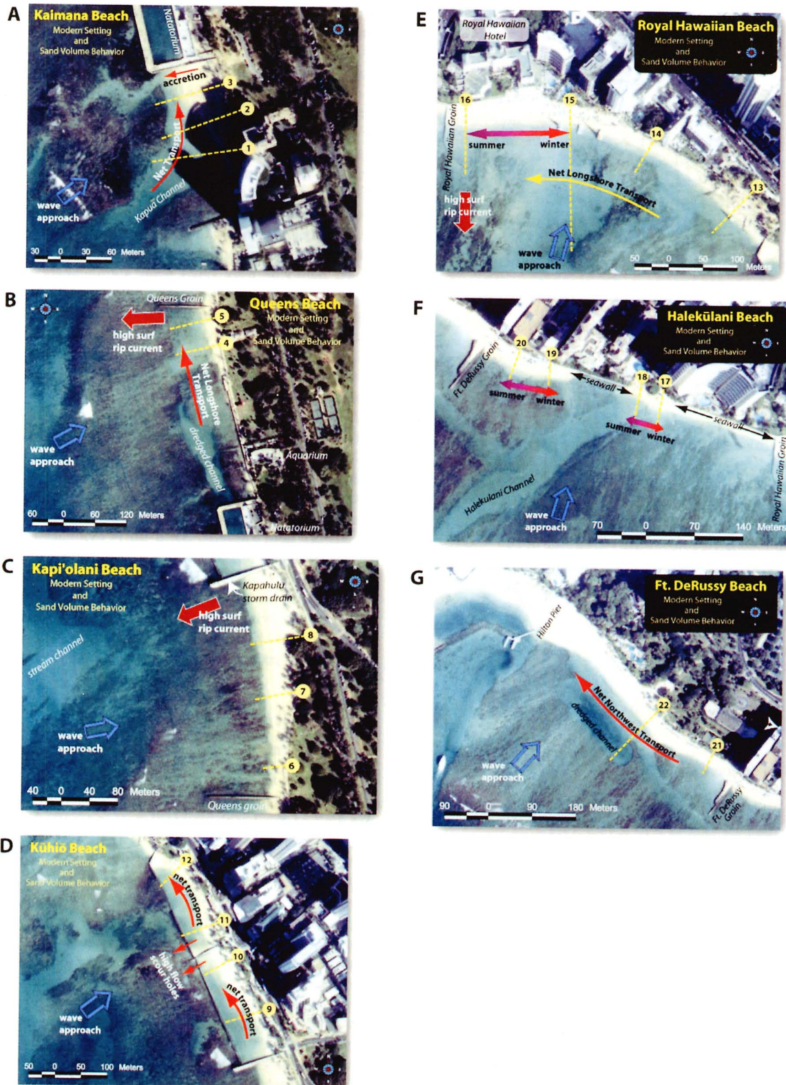
Figure 10A–G. Modern environmental setting and sand volume behavior by littoral cell, observed from beach profiles. (A) Kaimana Beach: Kapua Channel is an avenue for cross-shore transport. Net longshore transport is to the north, with accretion adjacent to the Natatorium at profile 3. (B) Queens Beach: Net longshore transport is to the north. Interruption of longshore currents by the Queens groin during high wave events can create an offshore rip, responsible for sand loss from the littoral cell. (C) Kapiolani Beach: Profile data indicate a stable setting. Interruption of longshore currents by the
