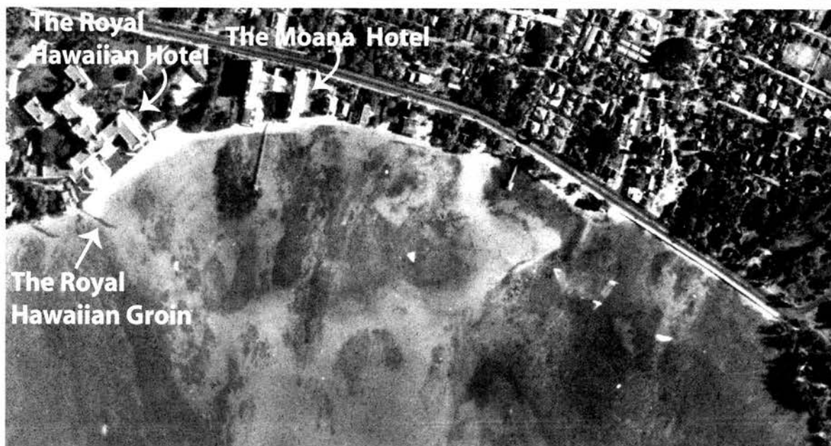
Figure 1. Waikiki Beach in 1927. The Royal Hawaiian Groin was one of 11 groins built along the beach between 1927 and 1930. It was reported to be the only groin successful in maintaining sand. However, downdrift starvation was caused to Halekulani Beach to the west. Note the wide beach fronting The Royal Hawaiian and Moana Hotels. The rest of the shoreline is without beach.
