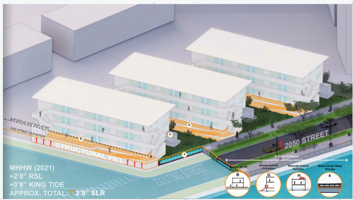
Figure 1: Site 1 retrofit for 2050 including building, transportation and open-space adaptation strategies with approximately 2'8" SLR.
