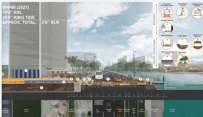
Figure 3: Site 2 retrofit for 2050 including building, transportation and open-space adaptation strategies with approximately 2'8" SLR.
