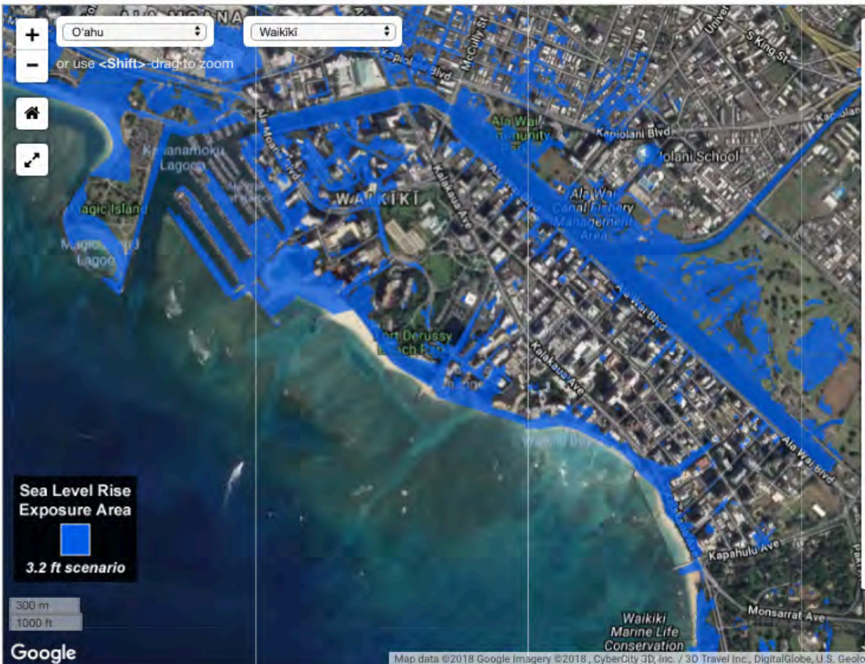
Figure 13. Results of Hawai'i Sea-Level Viewer showing the 3.2 ft SLR-XA for Waikiki. Results from: http://www.pacioos.hawaii.edu/shoreline/slr-hawaii/
