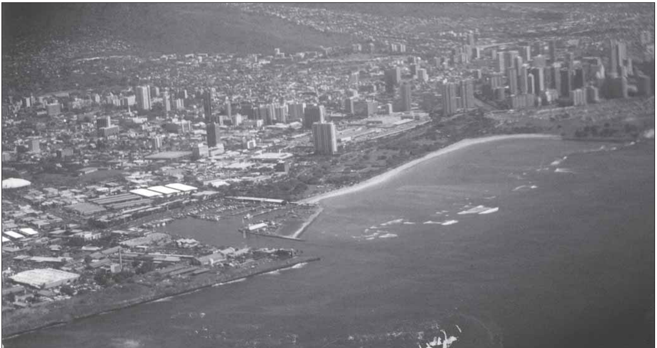
Figure 8. Kewalo Basin, Ala Moana Beach Park, Magic Island (Aina Moana); aerial photo, 19 January 1988. Note dredged channel in front of the man-made beach. (By R.L. Wiegel, #6354.)
